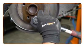
17 Remove the brake disc. Use a hammer.
