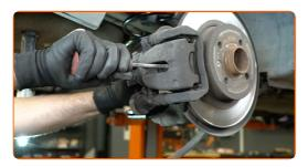
10 Remove the brake caliper.
