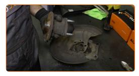
Treat the fasteners of the wheel hub bearing. Use copper grease.
