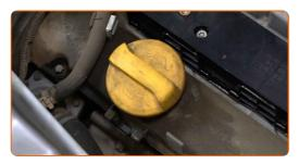
Unscrew the coolant reservoir cap.
