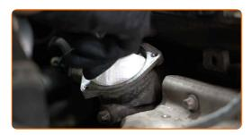
Clean the mounting seats of the thermostat housing. Use a seal scraper. Use all-purpose cleaning spray.
