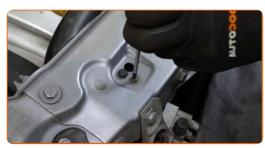
Remove the air distribution housing assembly.
