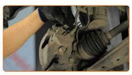
Install the brake caliper retaining spring. Use a flat screwdriver. Use pliers.
