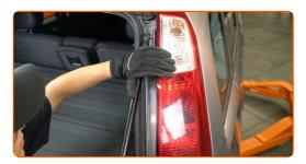
Snap on the circlip connecting the gas strut to the boot lid.
