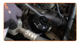
Unscrew the filter housing cap together with the old filter element. Use a drive socket #32. Use a ratchet wrench.
