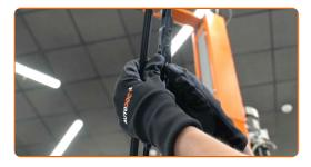
Remove the blade from the wiper arm.
