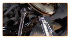
Screw the front arm fastener. Use a drive socket #18. Use a combination spanner #18. Use a torque wrench. Tighten it to 90 Nm torque.+75°
