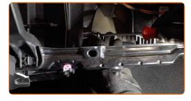
17 Install the air duct housing.
