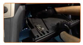
Remove the fasteners of the air duct housing.
