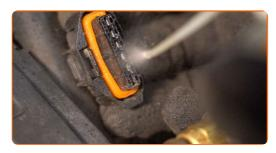
Plug in the ignition coil connector.
