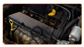
Take out the spark plugs. Use a telescoping magnet.
