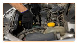
Tighten the ignition coil fastening. Use Torx T40. Use a torque wrench. Tighten it to 12 nm torque.
