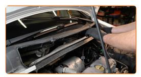
Screw in the fasteners of the lower part of the scuttle panel. Use a drive socket #10. Use a ratchet wrench.
