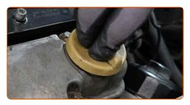
Tighten the oil filler cap.
