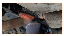
Unscrew the drain plug. Use Torx T45. Use a ratchet wrench.
