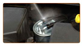
Disconnect the fuel supply lines from the fuel filter. Use fuel line pliers.
