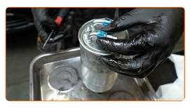
Remove the fuel pressure sensor.
