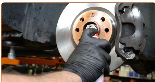
Replacement: brake discs – VAUXHALL Corsavan Mk IV (E) Van (X15). Tip:
