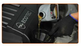
Replacement: engine oil and filter – VAUXHALL Corsavan Mk III (D) (S07). Tip from AUTODOC experts:
