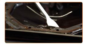
Clean the mounting seat of the transmission fluid pan gasket. Use a wire brush. Use cleaner&thinner.
