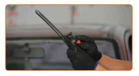
Remove the blade from the wiper arm.
