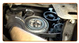
Place the V-ribbed belt on the tensioner pulley.
