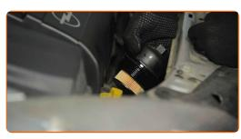
Use a drive socket #27. Use a torque wrench. Tighten it to 25 Nm torque.
