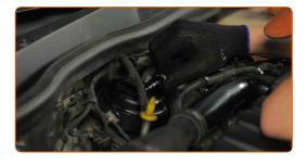
Attach the fuel pressure sensor connector.
