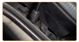
10 Remove the hydraulic transmission jack.
