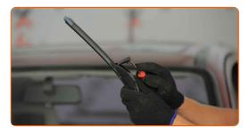
Remove the blade from the wiper arm.
