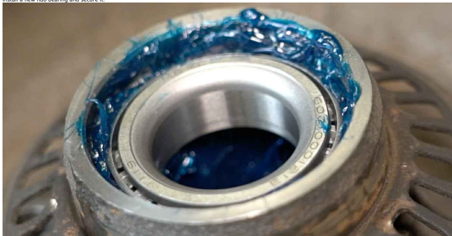
22 Install the wheel bearing oil seal.
