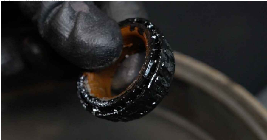
14 Clean the hub bearing mounting seat.
