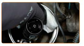
Install the cover of the oil filter housing and screw it on. Use a drive socket #32. Use a torque wrench. Tighten it to 15 Nm torque.
