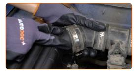
Screw the fastening clamp connecting the air duct to the air filter housing. Use a Phillips screwdriver.
