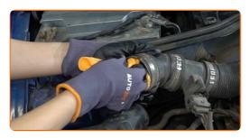
6 Release the air filter cover clips.
