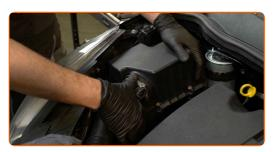
Screw in the fastening screws of the air filter cover. Use Torx T20. Use a ratchet wrench.
