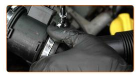
Screw in the fastener of the air intake pipe. Use Torx T25.
