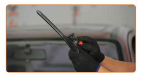
Remove the blade from the wiper arm.
