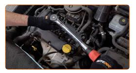
Replacement: spark plugs – VAUXHALL Corsa Mk II (C) Hatchback (X01). AUTODOC recommends:
