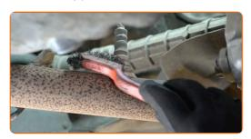
6 Unscrew the oxygen sensor fastener. Use a flare nut spanner #22.
