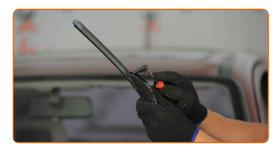
Remove the blade from the wiper arm.
