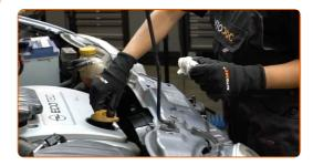
33 Tighten the oil filler cap.
