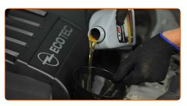
Replacement: engine oil and filter – VAUXHALL COMBO TOUR Mk II (C) (F25).
