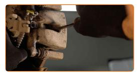
Remove the brake caliper. Use a crowbar.
