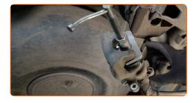
21 Install the brake caliper and fix it.
