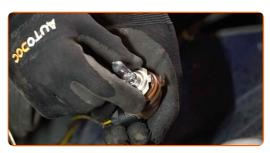
Replacement: headlight bulb – VAUXHALL Combo Mk III (D) Box Body / Estate (X12). AUTODOC recommends:
