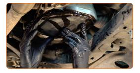
Replacement: manual gearbox oil – VAUXHALL Combo Mk III (D) Box Body / Estate (X12). Tip:
