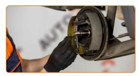
Insert retaining springs into pin slots. Use round-nose pliers. Use a flat screwdriver.
