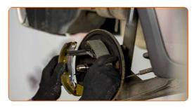
Install the brake pads retaining clips. Use round-nose pliers.
