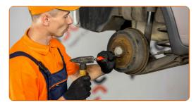
Replacement: brake shoes – VAUXHALL COMBO Mk II (C) Box Body / Estate (F25). Tip:
