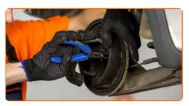
15 Remove the brake pads.
