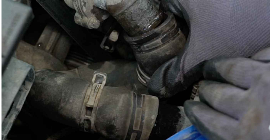
Replacement: engine thermostat - VAUXHALL Combo Mk I (B) Van (S93). AUTODOC recommends:
