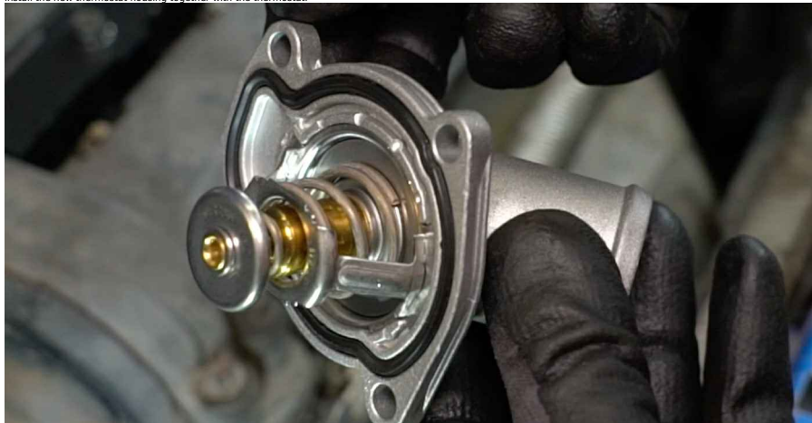
26 Install the rubber strip. 27 Tighten the thermostat housing fasteners. Use Torx T10. Use a torque wrench. Tighten it to 6 Nm torque.
