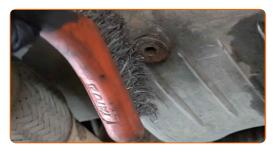
Unscrew the drain plug. Use HEX No.H7. Use a ratchet wrench.
