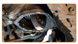
Replacement: manual gearbox oil – VAUXHALL Combo Mk I (B) Van (S93). Tip from AUTODOC:
