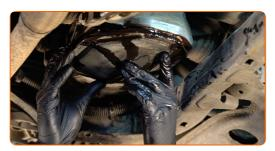
Replacement: manual gearbox oil – VAUXHALL Combo Mk I (B) Van (S93). Tip:
