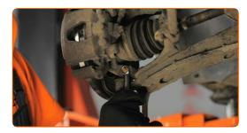
Remove the fastening bolt. Use a hammer.
