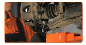
Treat the fasteners of the ball joint. Use copper grease.
