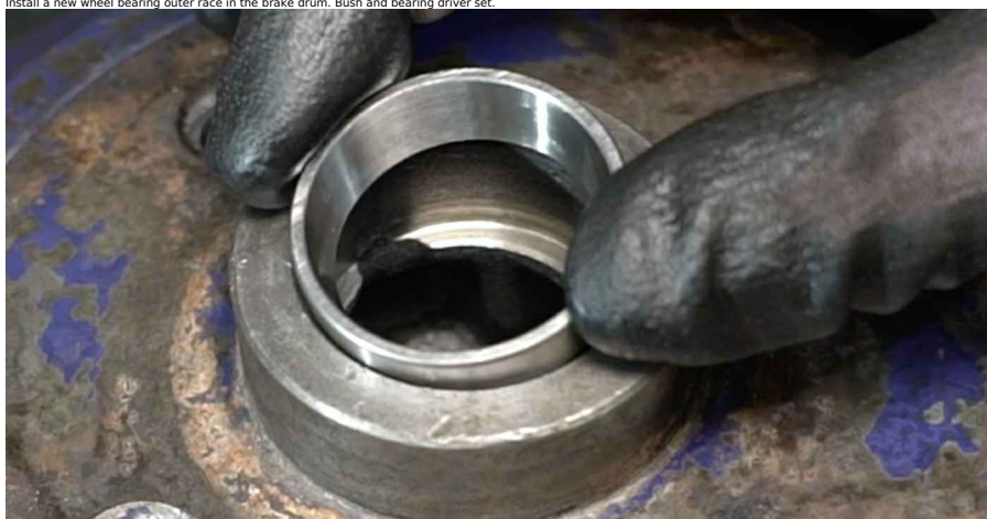
19 Install the new inner race of the wheel bearing into the brake drum. Bush and bearing driver set.
