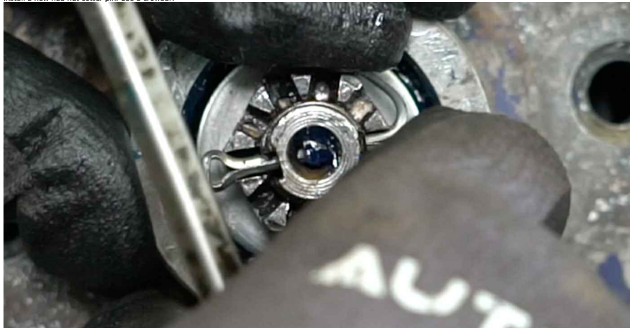
34 Install the cap of the hub nut. Use a rubber mallet.
