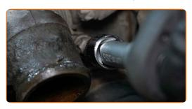
Remove the thermostat housing together with the thermostat.
