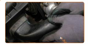
Attach the clip on the air filter intake hose.
