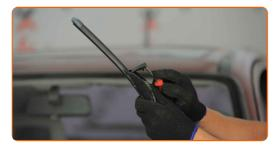
Remove the blade from the wiper arm.
