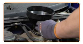
Pour coolant in the coolant reservoir.
