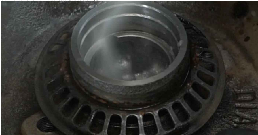
18 Install a new wheel bearing outer race in the brake drum. Bush and bearing driver set.
