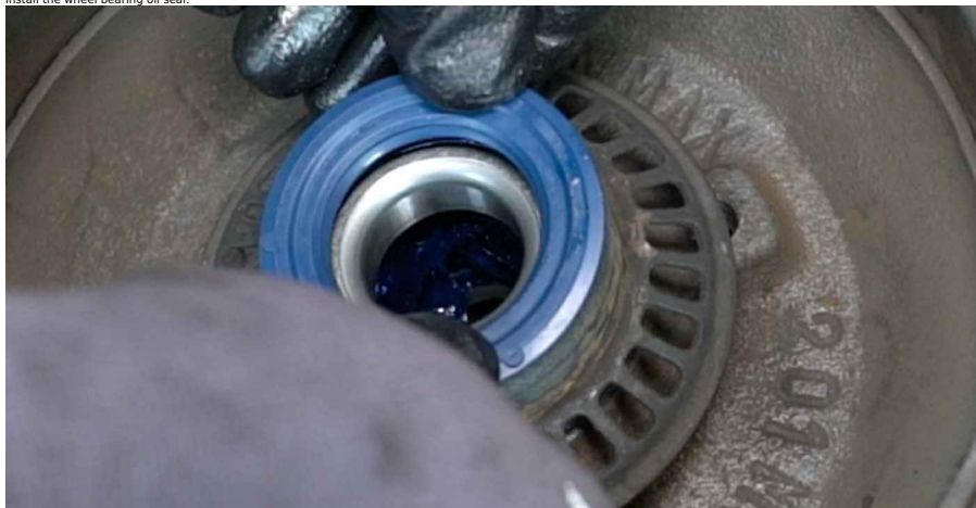
23 Treat the stub axle. Use all-purpose cleaning spray. Use bearing grease.
