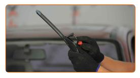
Remove the blade from the wiper arm.
