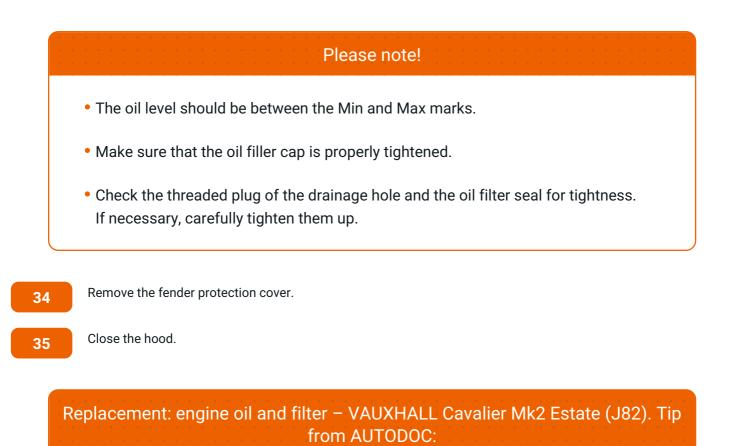
• Note that oil pressure warning light, which indicates insufficient pressure in the lubrication system, may be on for a longer time than usual. After a few seconds, the oil will fill all the channels, and the light will go out.
